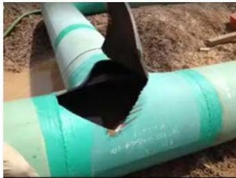
Since pressure testing of steel and copper piping systems is a regular occurrence in mechanical construction, it's important to guard against the complacency that sometimes accompanies performing pressure testing procedures over and over for long periods of time without incident. Most of the hazards associated with pressure testing result from the sudden, unintended release of stored energy. The risk of in-
